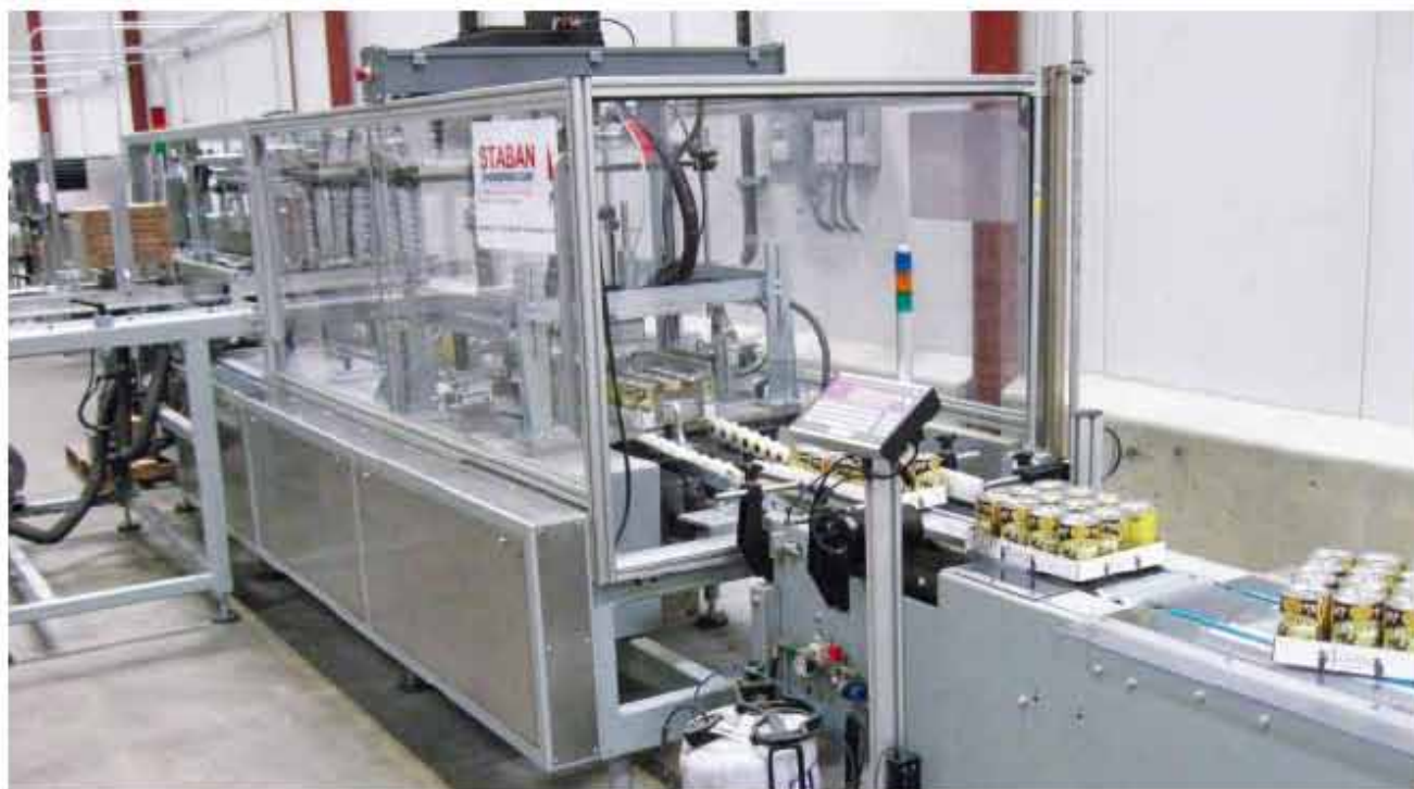
Trays leaving tray packer are turned 90 deg before traveling to stacker and then continuing to shrink wrapper.
