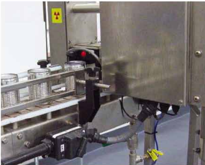
The packaging line runs through a monitor that checks for under-filled cans.
