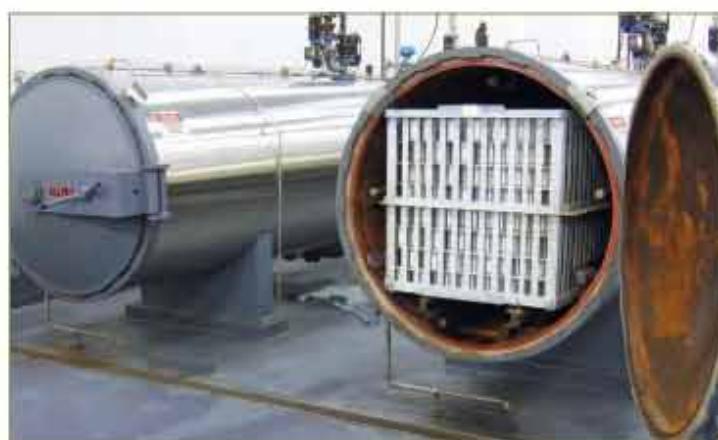
Four steam-heated retorts hold six crates of cans each.
