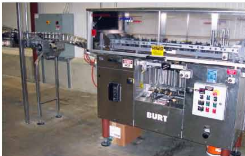
Roll-through labeler applies wraparound label to cans with hot-melt adhesive.
